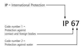
For safety reasons, connectors have to be protected against external influences like dust, foreign objects, direct contact, moisture and water. For industrial connectors, this protection is provided by their housings with their latching devices and sealed cable entries. The protection classes are also called IP Codes. The abbreviation IP stands for "ingress protection". Standard IEC 60529 specifies and divides the degree of protection into several classes.
