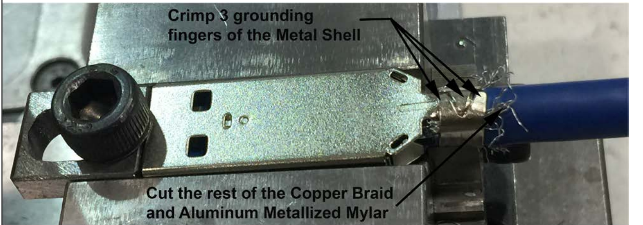
Figure 3-9: Terminate the USB Metal Shells
